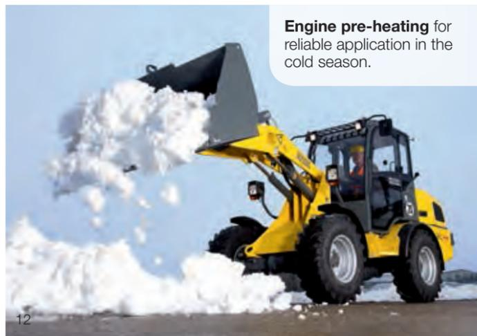
**High bucket breakaway force** for large volumes due to the Z-kinematics.
