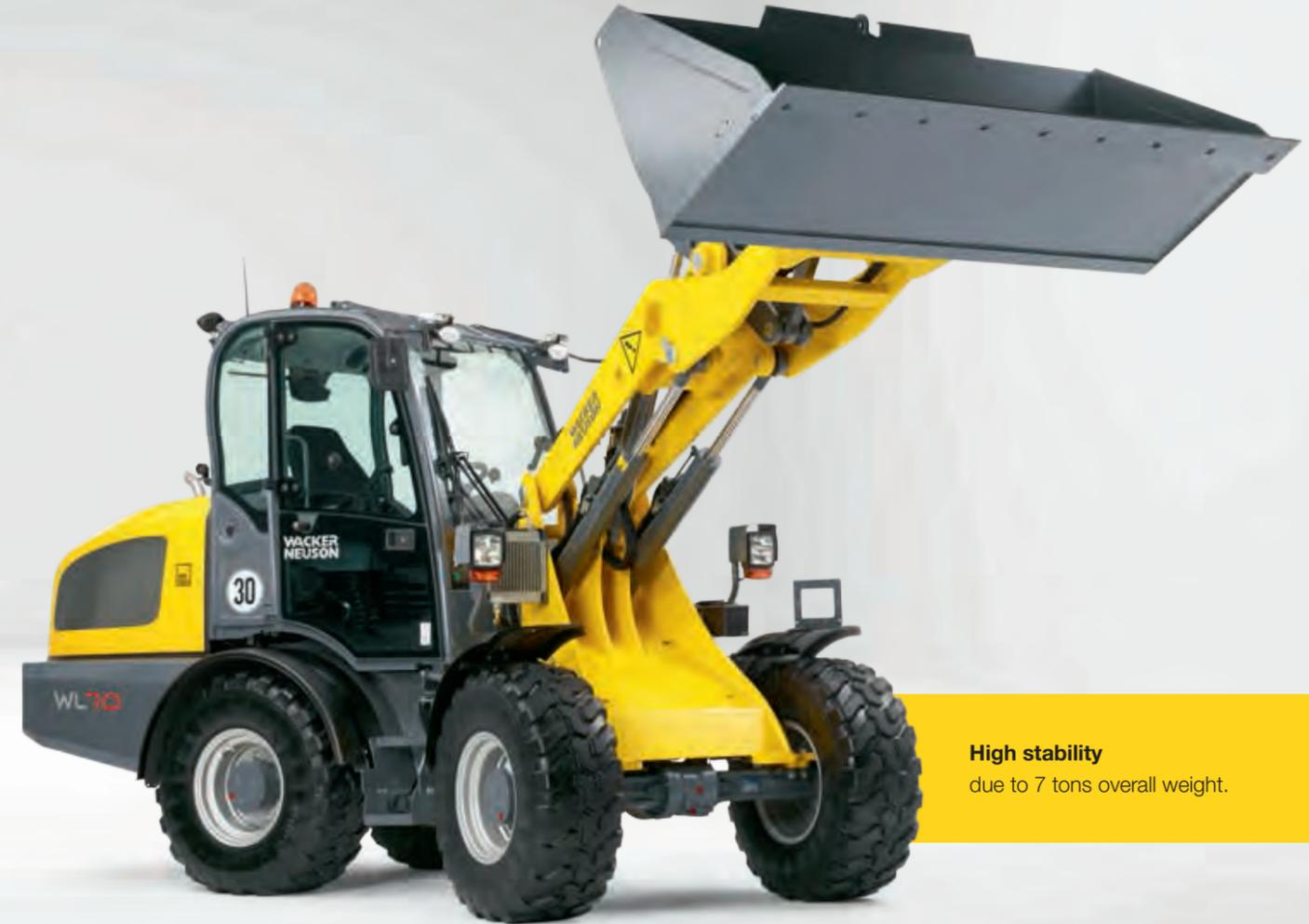
**High stability** due to 7 tons overall weight.
