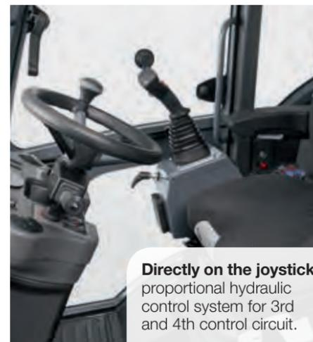
**Directly on the joystick:** proportional hydraulic control system for 3rd and 4th control circuit.
