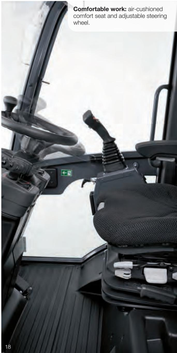
Adjustable joystick console swings along with the operator's seat.
