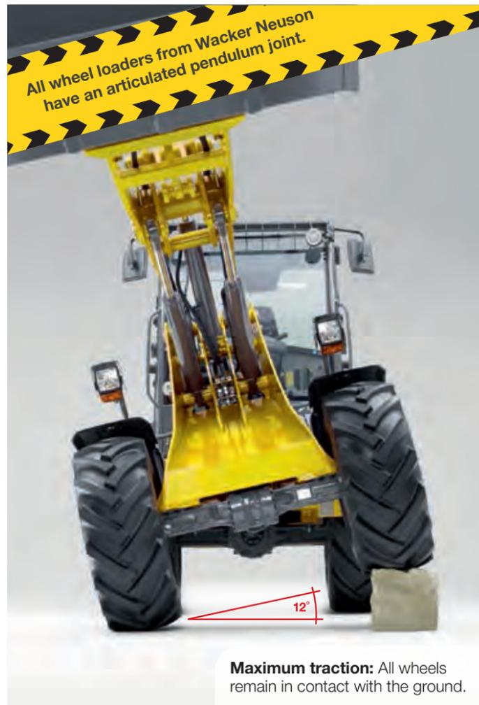
**Maximum traction:** All wheels remain in contact with the ground.
