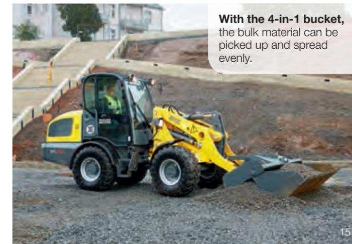
**With the 4-in-1 bucket,** the bulk material can be picked up and spread evenly.
